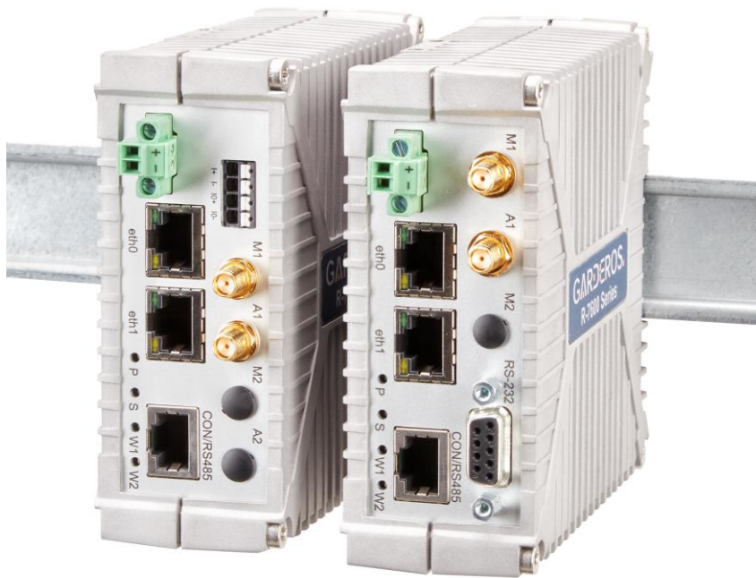
Fig. 1: Garderos R-7600 single radio routers optimized for smart grid.
